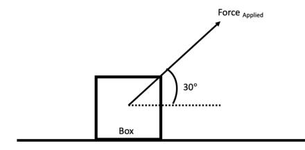
Now, looking just at the applied force, it can be broken into a horizontal and vertical component:
